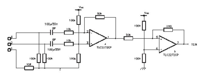
The LinCMOS amplifier outputs can drive rail to rail, making it also suitable for use as the comparator. Other types may be substituted provided that similar specifications are met. The shown circuit is biased to half the 5V power rail and comprises a balanced to single ended
