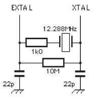
that part of the board layout. One of the capacitors may be changed to a trimmer type if higher precision than the crystal tolerance is required.
