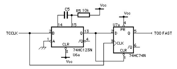
can output timecode while in fast forward or rewind-very fast speeds may result than produce a large interrupt load. The following circuitry may be used to limit reading to a speed no greater than double normal playspeed:
