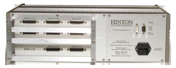
The MIDIX-30 rear is divided into two panels: The MIDI I/O panel and the MIDIX Controller panel.
