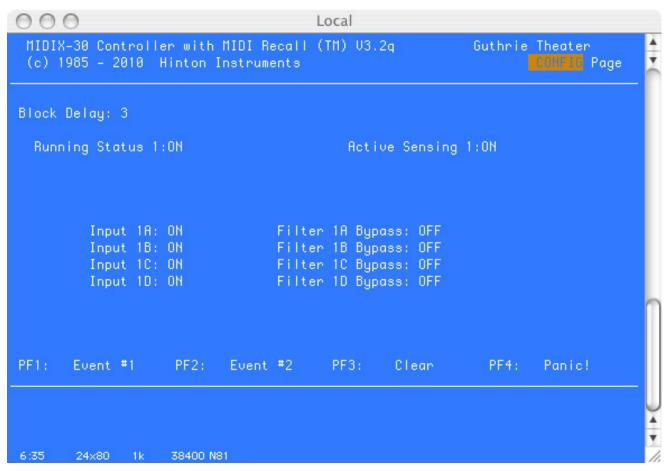
**Block Delay:** 0 - 9, sets the delay between large generated blocks of data to prevent overflowing the data buffers of receiving equipment.
