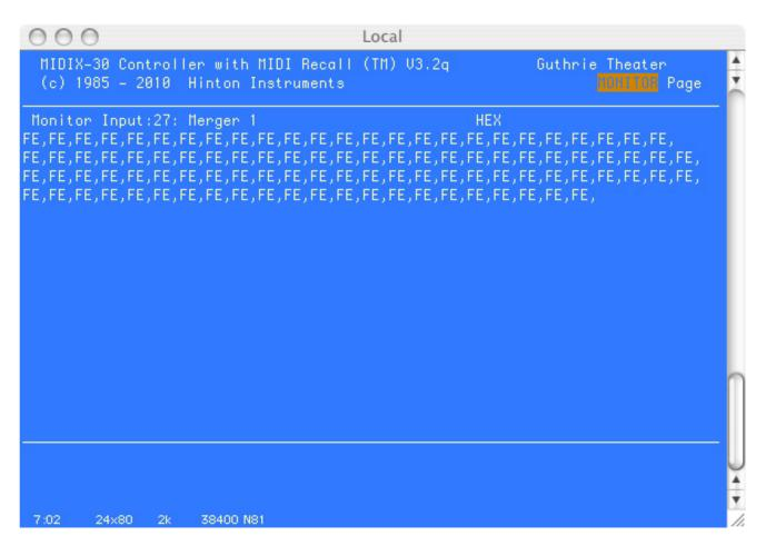
Monitor Source: Input 1-30, selects the matrix Input to Monitor.
